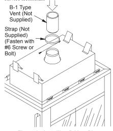
Figure 9 - Installing B-Vent Pipe
